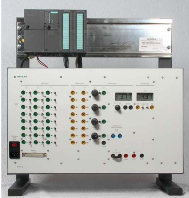
SIMATIC Experimental Rack W4734-1E CPU 314C-2PN/DP, 24DI, 16 DO, 5 AI, 2AO
